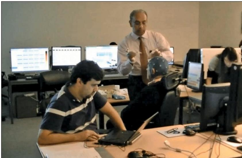
Hussein Abbass at Eurocontrol Experimental Centre, Brétigny, France, injecting gel into an EEG electrode while preparing a participant before an augmented cognition experiment.
