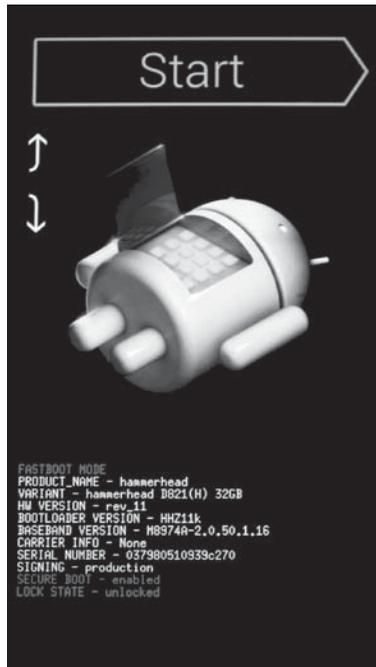
Figure 13-1: Nexus 5 bootloader screen
